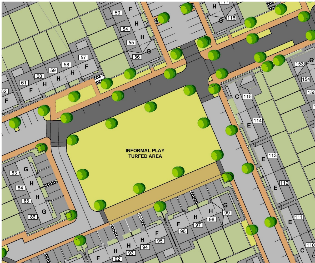
Figure 13: Showing area where a variety of different forms of parking are provided, with on-curtilage parking, and shared parking both perpendicular and parallel to reduce impact, with landscaping included.
